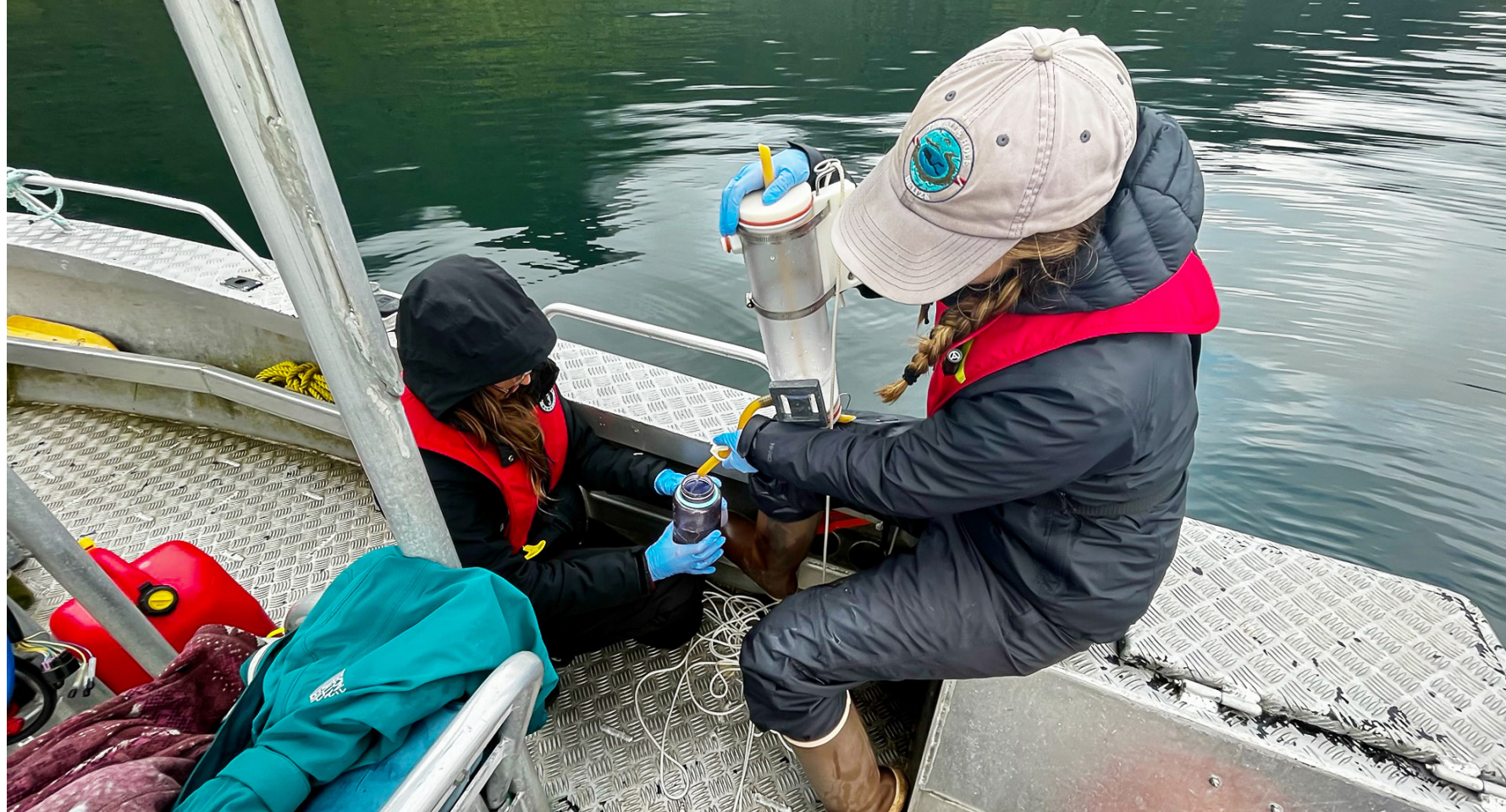
The premise of eDNA is that organisms leave a genetic trace in the aquatic environment that can be detected by the collection, filtering and DNA screening of water samples.
